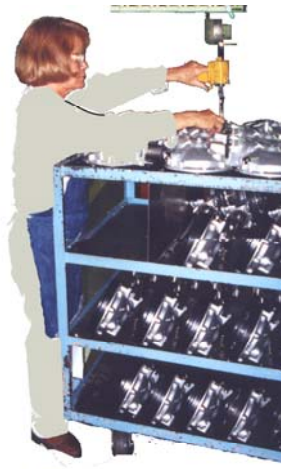
Figure 3. Batch method of oil filling
